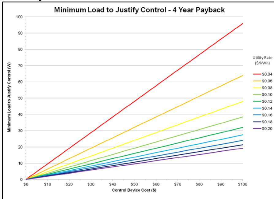
Figure B-3 Minimum load that can be cost-effectively controlled by a control device – 4-year payback (Credit: Chad Lobato/NREL)
