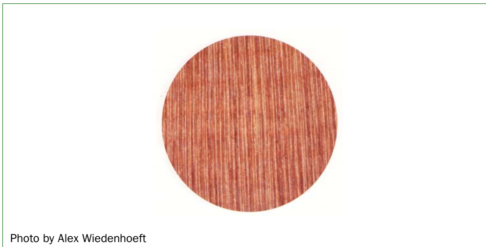
FIGURE F-2 Example of Araucaria araucana (Monkey puzzle tree) Wood Cross Section
