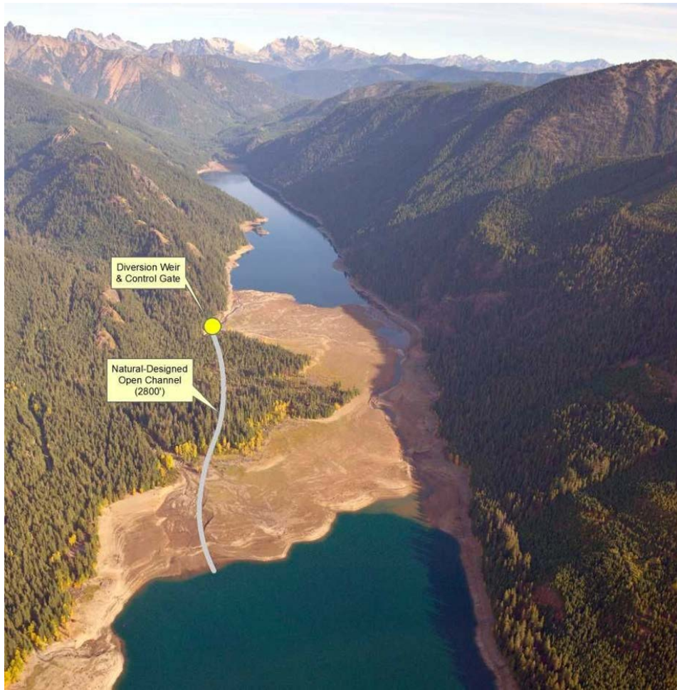
Figure 9-31. OPTION 6 - The Narrows: Lower to Upper Reservoir Passage -Natural Channel conceptual design.
