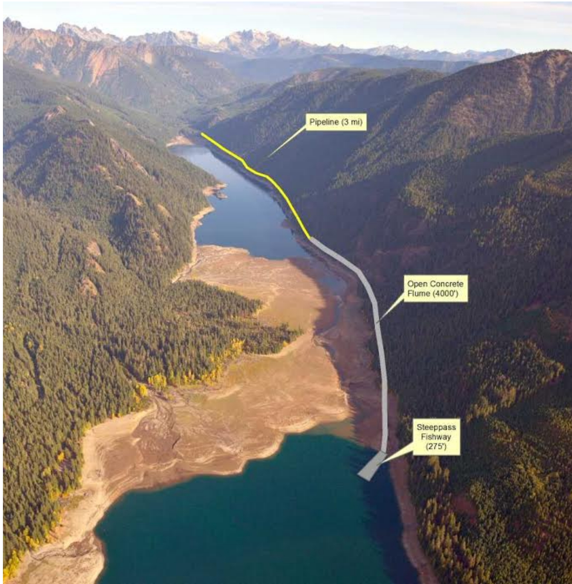
Figure 9-29. OPTION 4 - The Narrows: Lower to Upper Reservoir Passage - Gravity Flow from Mineral Creek conceptual drawing.
