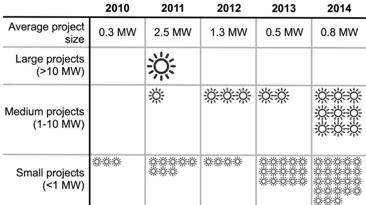
**Figure 13. Schematic of community solar array size from 2010 to 2014**
