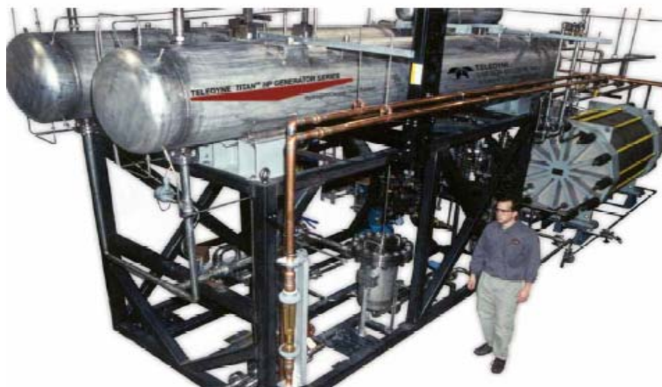
Figure 8: The TELEDYNE TITAN™ HP Generator Series produces ultrapure, pressurized hydrogen without the need for additional purification. 38
