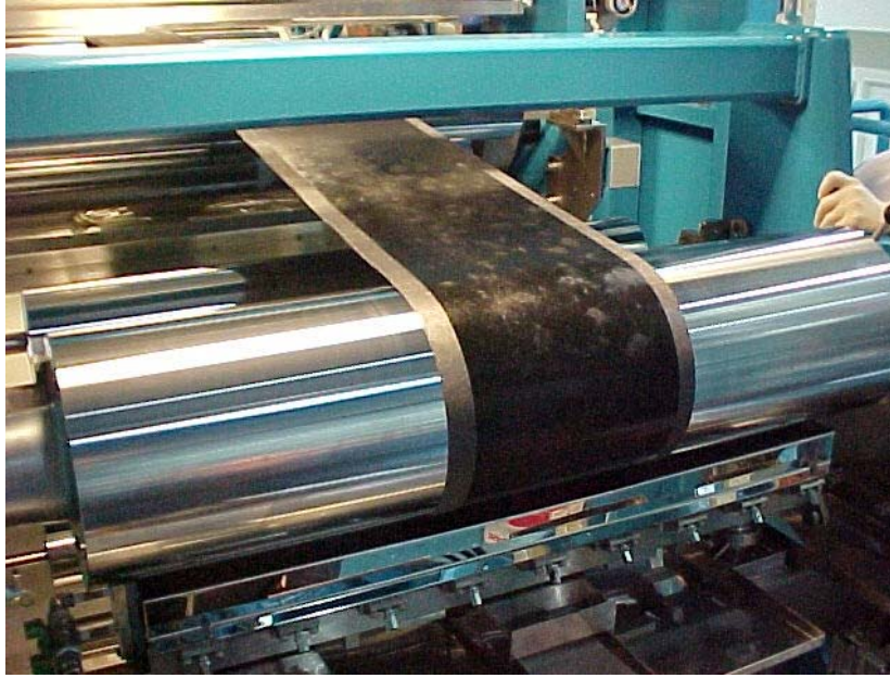
Figure 6: Semi-automated discrete/continuous fabrication of catalyst coating. 30
