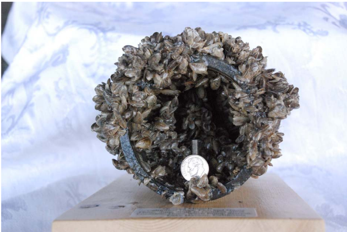
Pipe encrusted with zebra mussels. (Photo: California Department of Fish and Game)
