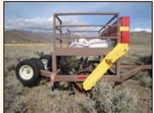
Lawson Aerator. Teeth on the cylinder aerate the soil to prepare a seedbed. A seed box attached to the aerator distributed native grass and forb seeds.
