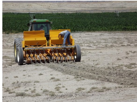
Dean on the back of a drill seeder making sure everything flows properly.
