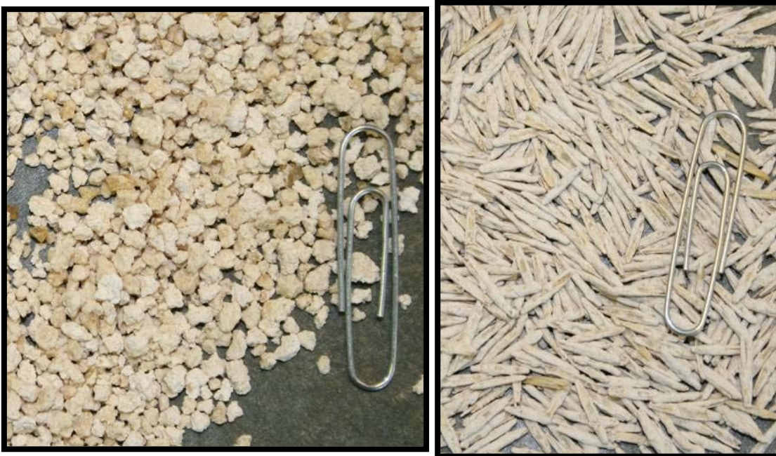
Figure 1. Zeba Farm soil amendment (left) and used as a seed coating (right).
