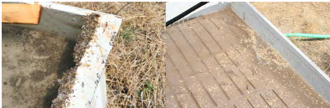
Figure 4. Loose Fertil Fibers (l) and rice hulls (r) washing off of the plots.
