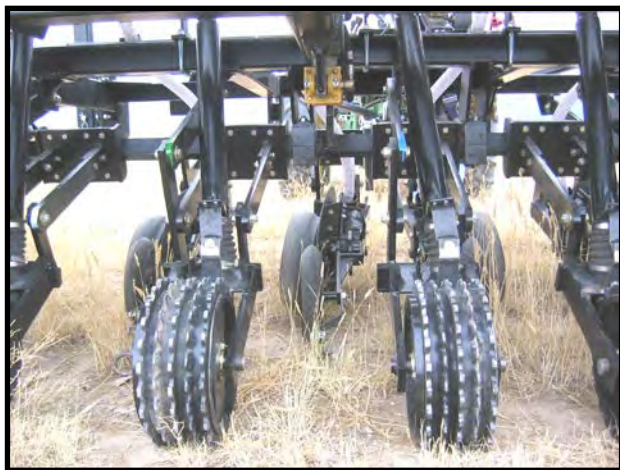
Photo 2.5. Addition of broadcast seeders to alternate rows of drilled and broadcast seeds to facilitate planting shallow-seeded species and deep-seeded species in a single operation.
