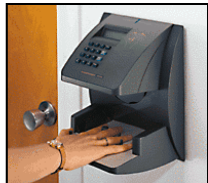
Access Control Terminal
