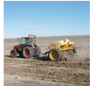
Rangeland drill used for site preparation and seed placement. (Photo: USFS, 2006)
