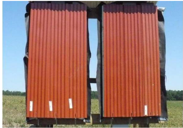
Figure 22. Lightweight cladding panel installed over the test wall assemblies
