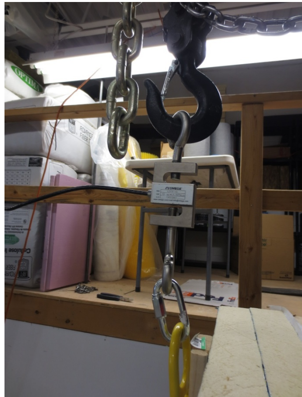
Figure 18. Load cell installed between furring strip and hoist
