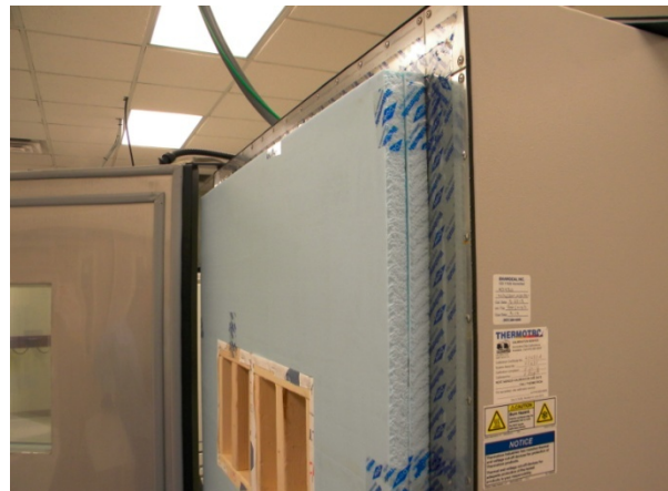
Figure 16. Assemblies installed in climate chamber opening
