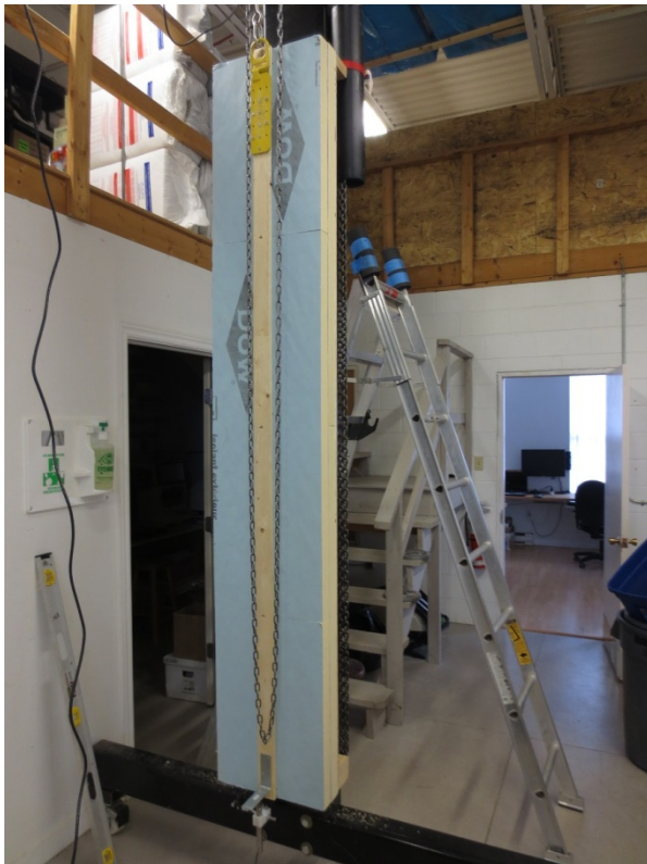
Figure 17. Full height deflection test assembly
