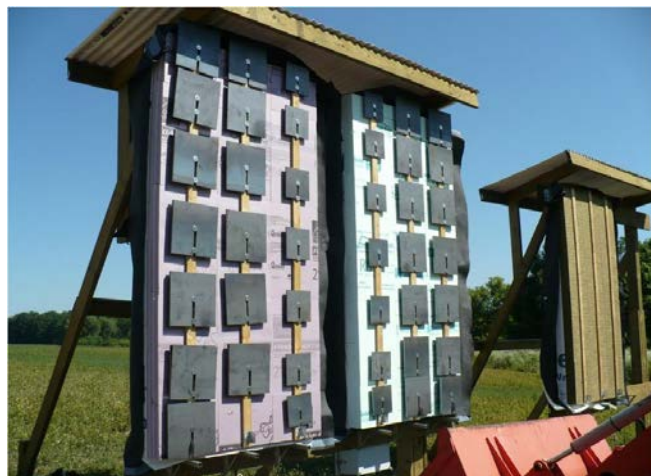
Figure 21. Exposed wall assemblies loaded to representative cladding weights
