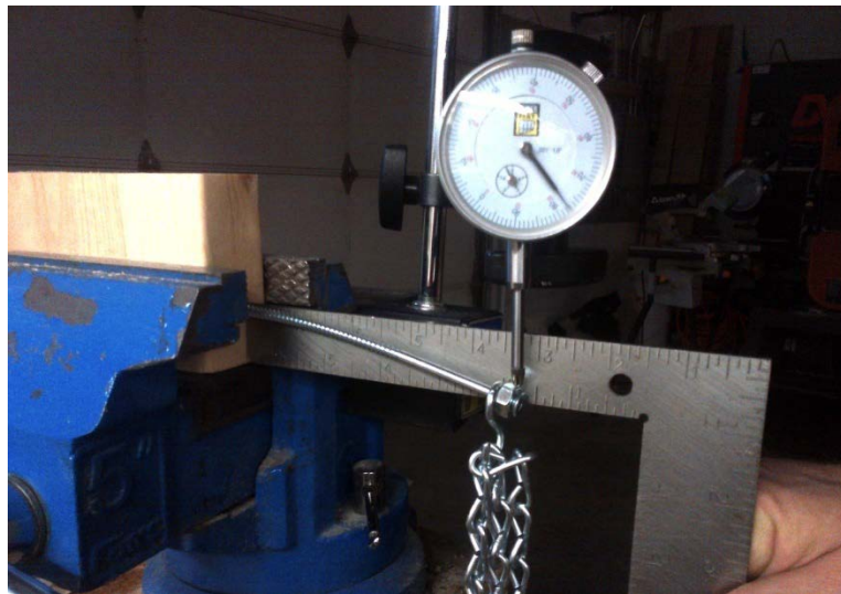
Figure 28. Simple screw cantilever bending test
