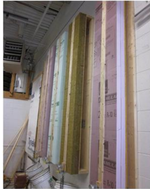
Figure 6. Long-term gravity load response test setup
