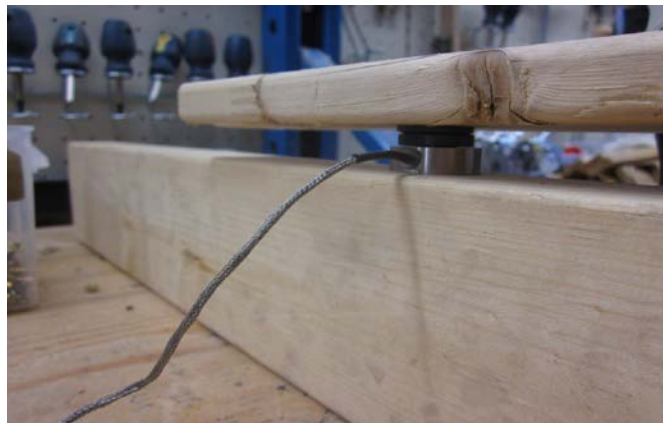
Figure 15. Precompression force test setup
