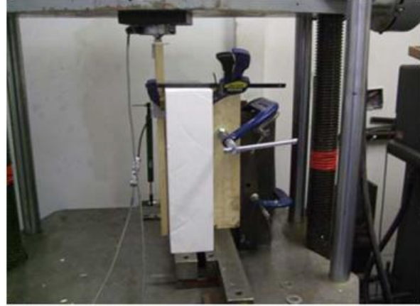
Figure 2. Typical ASTM D1761 test setup
