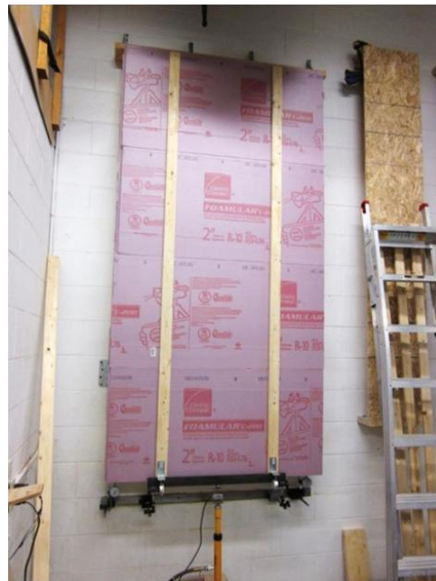
Figure 3. Short-term gravity load response test setup
