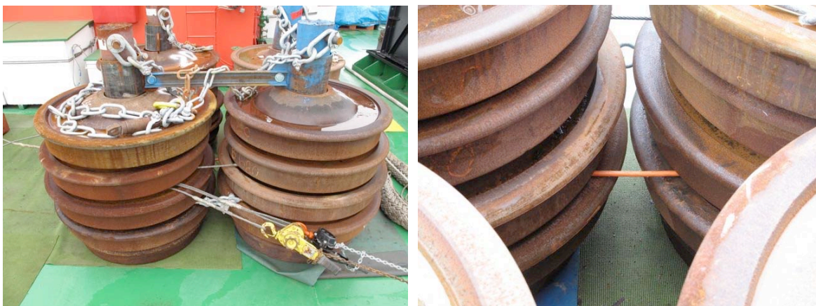
Note the coated wire rope binder around the lower part of the anchor.
