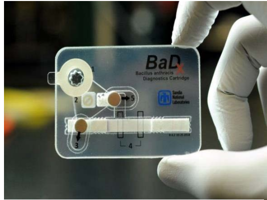
BaDx (Bacillus anthracis Diagnostic) Cartridge - also known as Anthrax Detection Cartridge
