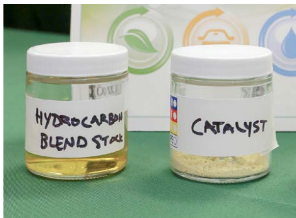
Samples of drop-in replacement gasoline produced using ORNL's catalytic ethanol upgrading technology
