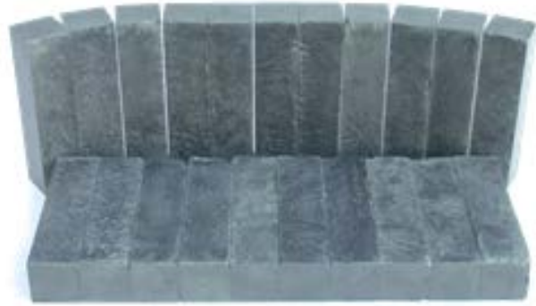
Sulfur concrete bricks made using the SSBAF process
