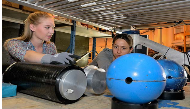
Researchers prepare a lead hemisphere inside a muon tomography machine, which can peer inside closed containers and provide detailed images of dense objects, such as nuclear materials, or other items of interest.
