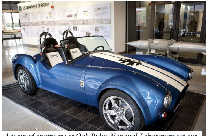
A team of engineers at Oak Ridge National Laboratory set out to create a replica of this iconic car using a massive 3D printer, advanced composite materials, and exciting new electric vehicle technologies.
