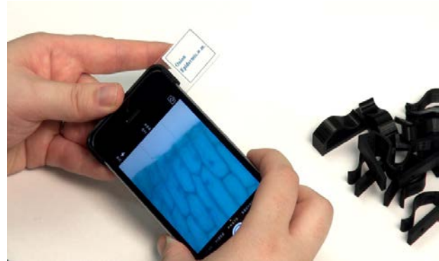
3D-printed microscope attached to a cell phone shows the epidermis of an onion magnified 350 times.
