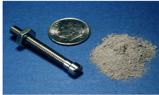
Titanium bolt made from 1.8 grams of gas atomized titanium powder
