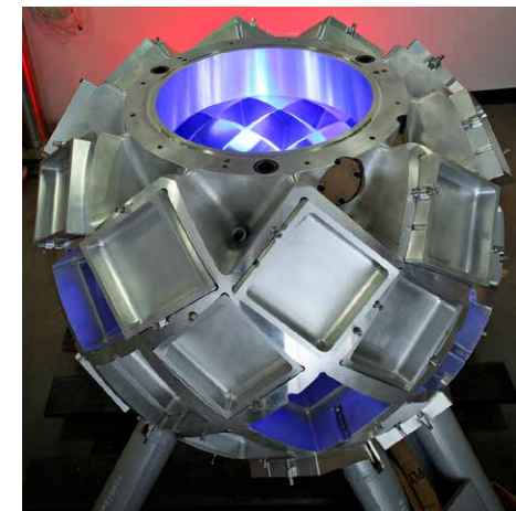
Detector Array for the TOPAZ Single-Crystal Diffractometer at the Spallation Neutron Source at Oak Ridge National Laboratory.
