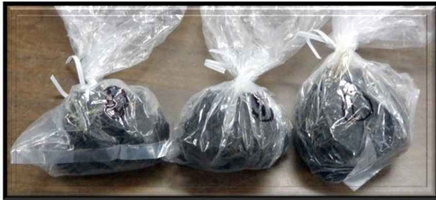
Figure 10.—Clod bags that have been correctly sealed with a twist tie. (Step 22)
