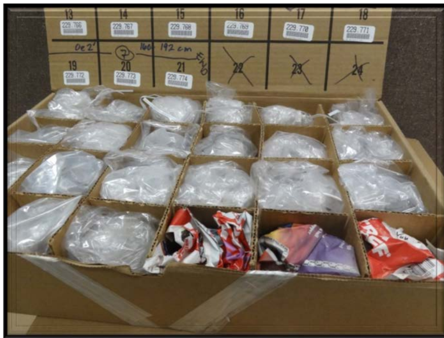
Figure 11.—A clod box in which the empty cells have been filled with packing material to increase stability. (Step 24)
