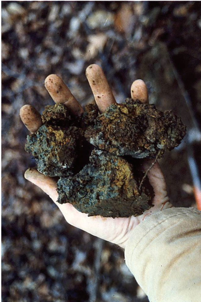
Figure 49. —Glauconitic soils typically have gleyed, green, or black matrices and can have mottles of weathered sulfides that can be mistaken for redox concentrations. If the weathered sulfides in this glauconitic soil were mistaken for redox concentrations, this nonhydric soil would appear to meet the requirements of indicator F6 (Redox Dark Surface).
