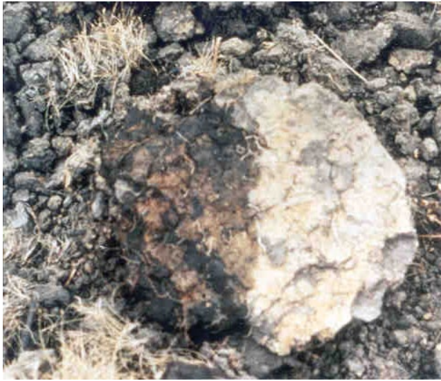
Figure 3. —The left portion of this ped shows moist soil colors, and the right portion shows dry soil colors. Moist colors are to be used when hydric soils are identified. The moist colors in this picture would meet the requirements for indicator F6 (Redox Dark Surface), but the dry colors would not meet these requirements.
