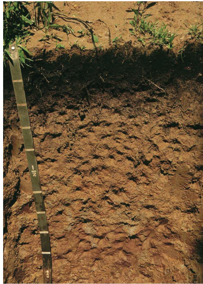
Figure 39.—Indicator F20 (Anomalous Bright Loamy Soils). This indicator is restricted to areas near estuarine marshes or water. It does not require a matrix color with chroma of 2 or less.
