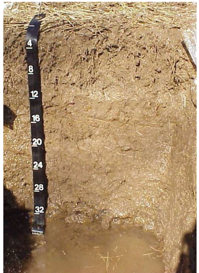
Figure 41.—Indicator F3 (Depleted Matrix) in red parent material. If a soil that formed in red parent material stays wet and anaerobic long enough, it may develop the indicator F3.
