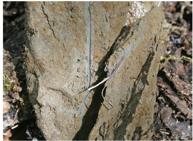
Figure 20.—Indicator A15 (Alaska Gleyed Pores). Gleyed colors are along root channels. Reduction occurs first along root channels, where organic carbon is concentrated.
