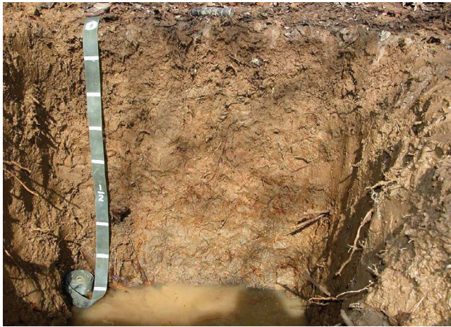
Figure 38.—Indicator F19 (Piedmont Flood Plain Soils). This indicator is restricted to active flood plains. It does not require a matrix color with chroma of 2 or less.
