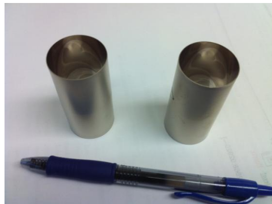
Fig. 1: Pure nickel mirrors electroformed using pulse plating technique
