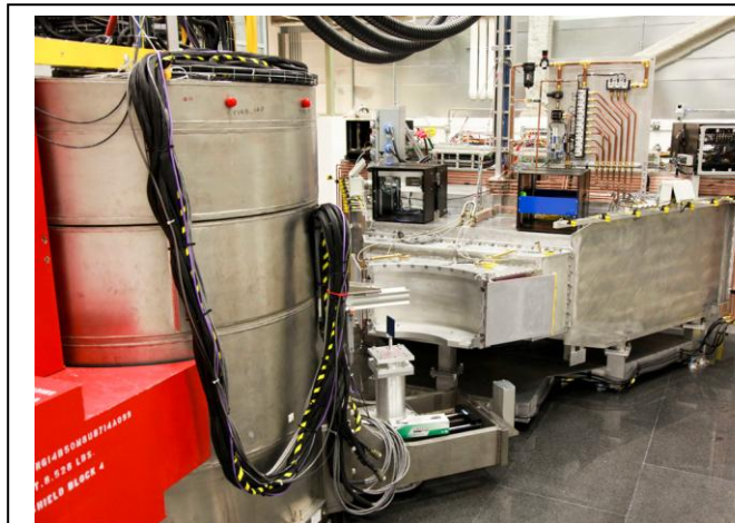
Figure 2. Photograph of the HYSPEC secondary spectrometer – the focusing crystal drum shield, the sample stage and the detector vessel – in the satellite building.
