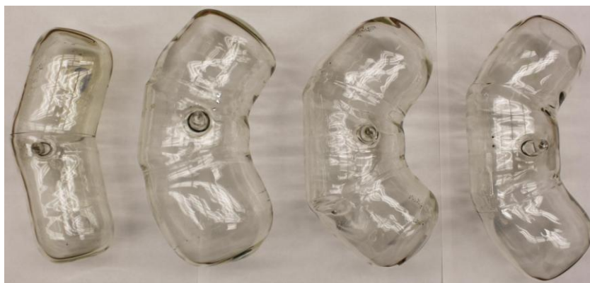
Fig. 1. SEOP spin filter cells for wide-angle polarization analysis.
