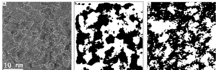
Figure 1 Comparison of (a) the original HRTEM image with hand-drawn c/a boundaries; (b) simulated c/a morphology by coarse-grained modeling ;(c) the experimental image (a) after processing. In (a) the c/a boundaries are shown as white dashed lines, in (b) and (c) white and black colors represent crystalline and amorphous regions, respectively.
