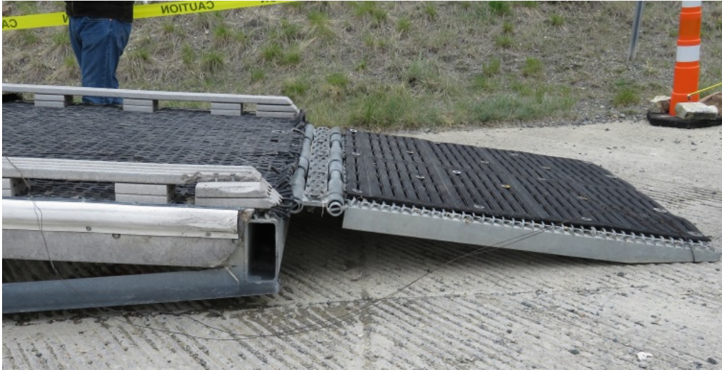
Figure 3: Access Ramp, open as if for use.
