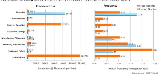
The leading event type affecting crude oil pipeline and petroleum product pipelines in Utah during 1986 to 2014 was Equipment Failure for crude oil pipelines and Corrosion for product pipelines, with an average 0.24 and 0.18 incidents per year (or one incident every 4.1 and 5.7 years), respectively.
