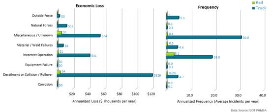
The leading event type affecting the transport of petroleum product by rail and truck in Ohio during 1986 to 2014 was Incorrect Operation for rail transport and Miscellaneous/ Unknown for truck transport, with an average 3.1 and 30.8 incidents per year, respectively.
