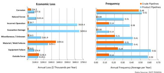
The leading event type affecting crude oil pipeline and petroleum product pipelines in Ohio during 1986 to 2014 was Corrosion for crude oil pipelines and Equipment Failure for product pipelines, with an average 0.48 and 0.62 incidents per year (or one incident every 2.1 and 1.6 years), respectively.
