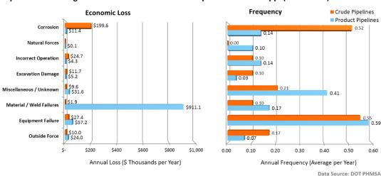
The leading event type affecting crude oil pipeline and petroleum product pipelines in Mississippi during 1986 to 2014 was Equipment Failure for crude oil pipelines and Equipment Failure for product pipelines, with an average 0.55 and 0.59 incidents per year (or one incident every 1.8 and 1.7 years), respectively.
