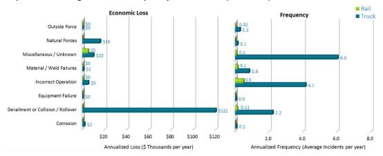
The leading event type affecting the transport of petroleum product by rail and truck in Mississippi during 1986 to 2014 was Incorrect Operation for rail transport and Miscellaneous/Unknown for truck transport, with an average 0.5 (or one incident every 2 years) and 6.0 incidents per year, respectively.
