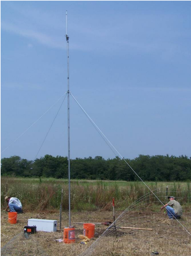
Pictured above is one of four semi-permanent dipole (unidirectional) antenna stations equipped with automatic data-loggers. The four towers provide complete coverage of the study area 24/7 to determine presence/absence of radio-marked birds during the hunting season.
