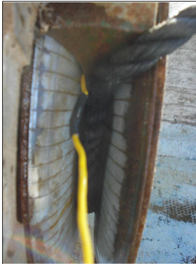
Figure 2-6 Tag Fouling Under Winch Pulley Ejection Device
