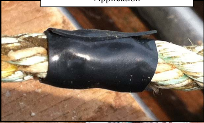
UHF Tags Directly after Application
