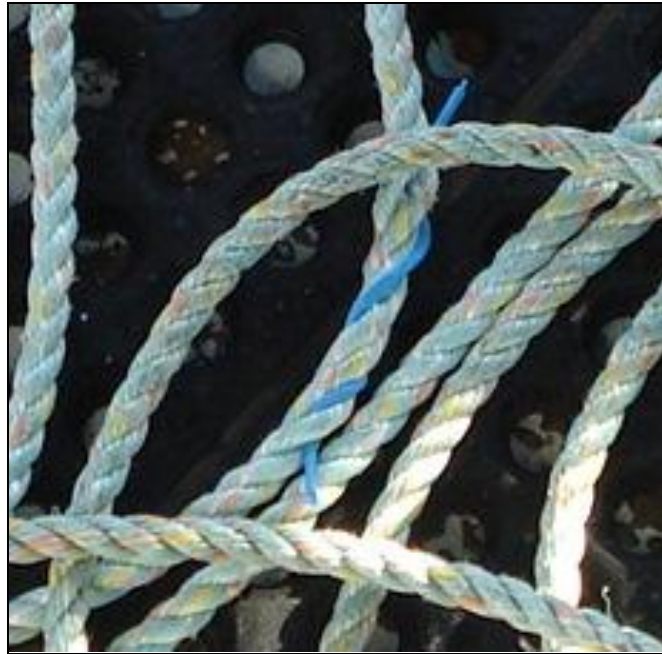
Figure 2-2 Example of Woven Tag Inserted into Line
