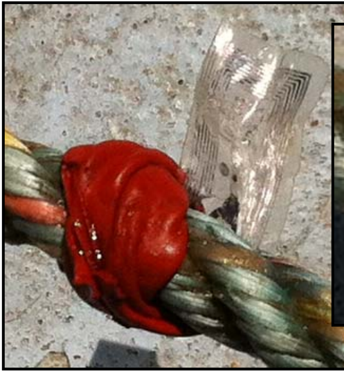
NFC Tag after Run 17 – Only Red NFC Tag Exhibiting Any Change in Backing Properties
