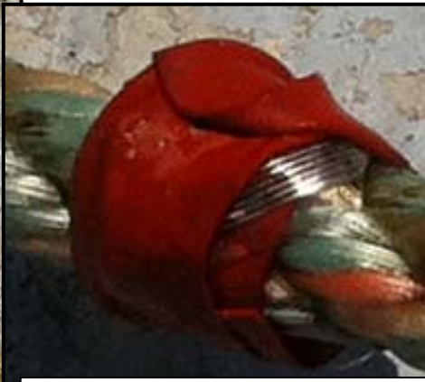
NFC Tags after Run 21 – Run 21 Caused the Rope to Drag Across a Surface that Destroyed the Backing on Every Tag
