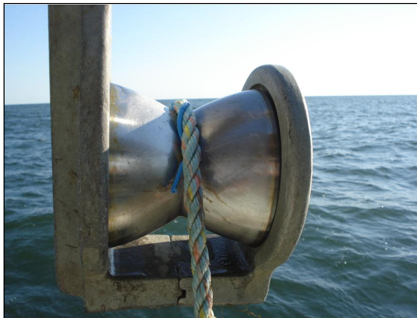
Figure 2-3 Tag Woven into Line Traversing a Line Guide
