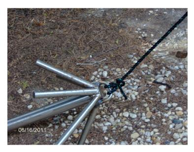
New eye welded on grappling anchor to make handling easier and safer
