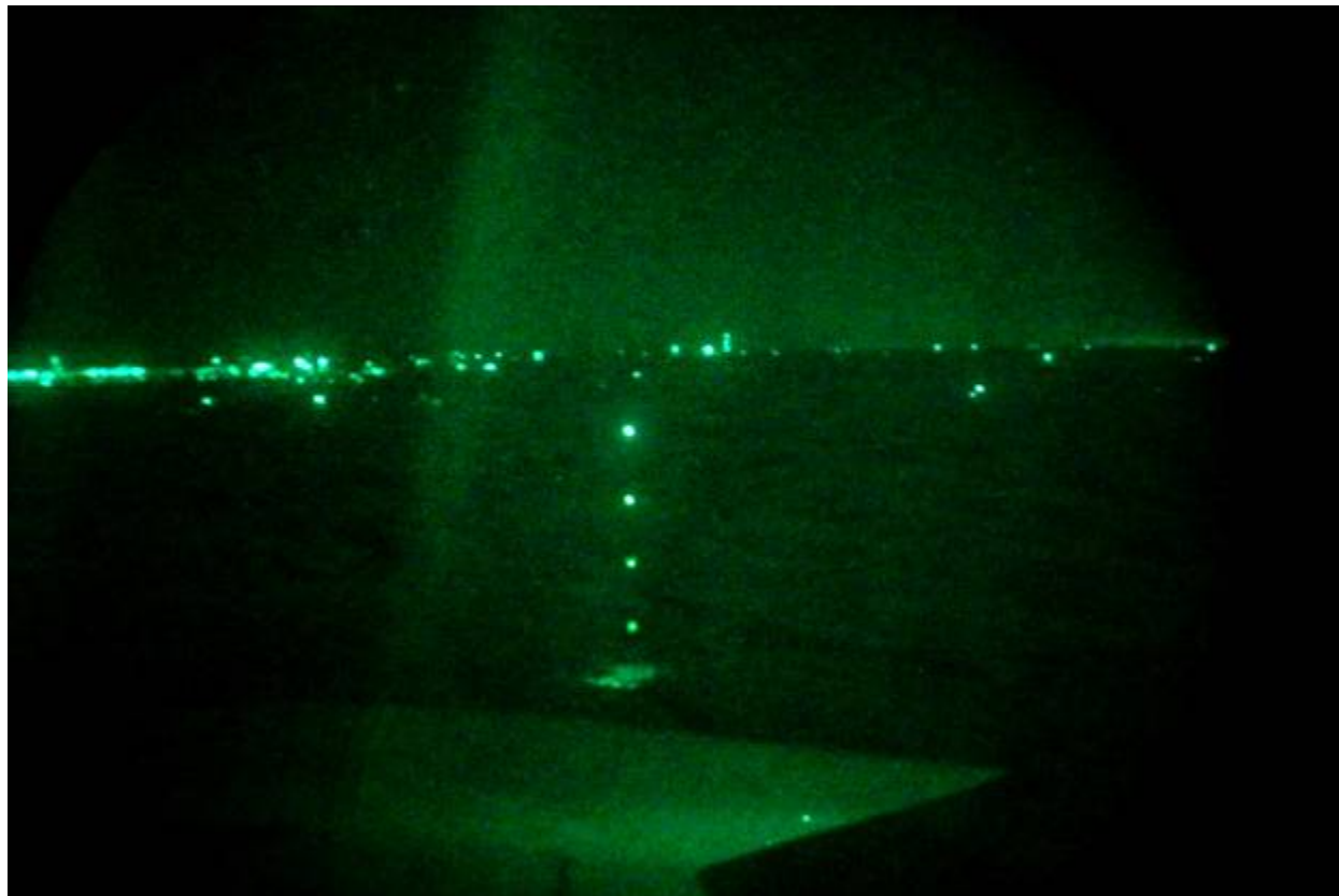
Figure 9. View of the WPBN Tower Without L-810s Through a Night Vision Scope
