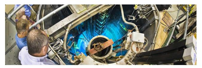
At the Annular Core Research Reactor (ACRR) facility, Sandia researchers can subject various test objects to a mixed photon and neutron irradiation environment featuring either a very rapid pulse rate or a long-term, steady-state rate. ACRR has operated since 1979.
