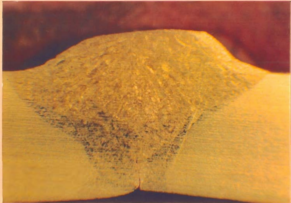
Figure 3 Apparent Lack of Penetration in Longitudinal Weld
