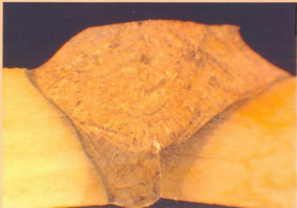
Figure 4 Incomplete Penetration in Longitudinal Weld
