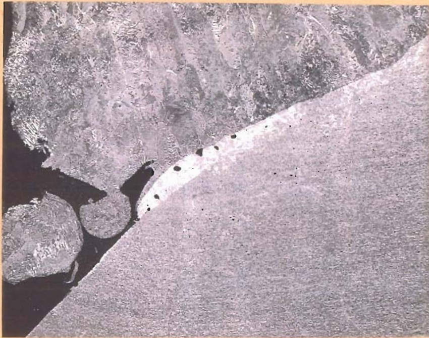
Figure 11 Close-up View of Previous Defect, 25X
