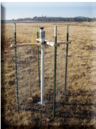
Shallow Ground Water Well-Monitoring System
