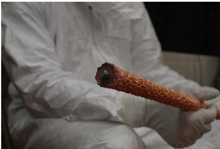
Figure 2: Electroformed copper part that will become part of the MJD module.
