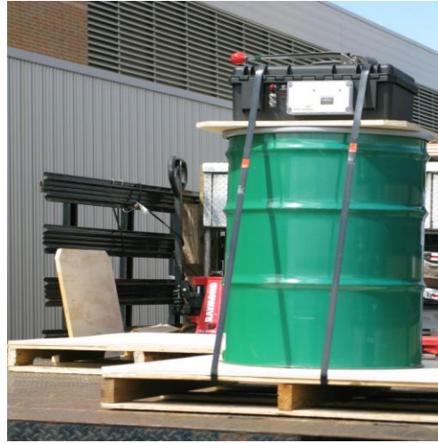
Figure 5: The \mu -Witness detector attached to one of the steel drums used to transport the electroformed copper during shipment from PNNL to SURF.
