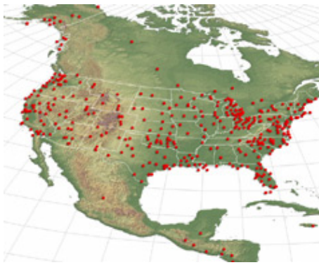
The Continuously Operating Reference Stations (CORS) system is a network that continually corrects GPS signals, and provides these corrections to GPS users over the Internet. Click on the image for larger view.
