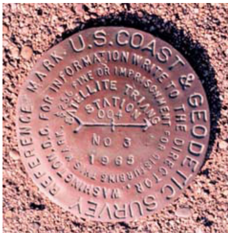
Brass monuments permanently affixed in concrete or surrounding bedrock indicate accurate geodetic reference positions within the National Geodetic Survey's horizontal and/or vertical datums. Click on the image for larger view.
