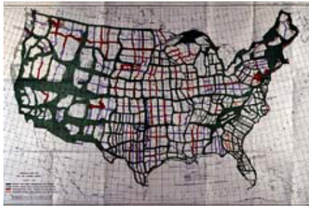
A United States triangulation network map from 1937. This system was a precursor to today's modern National Spatial Reference System. Click on the image for larger view.
