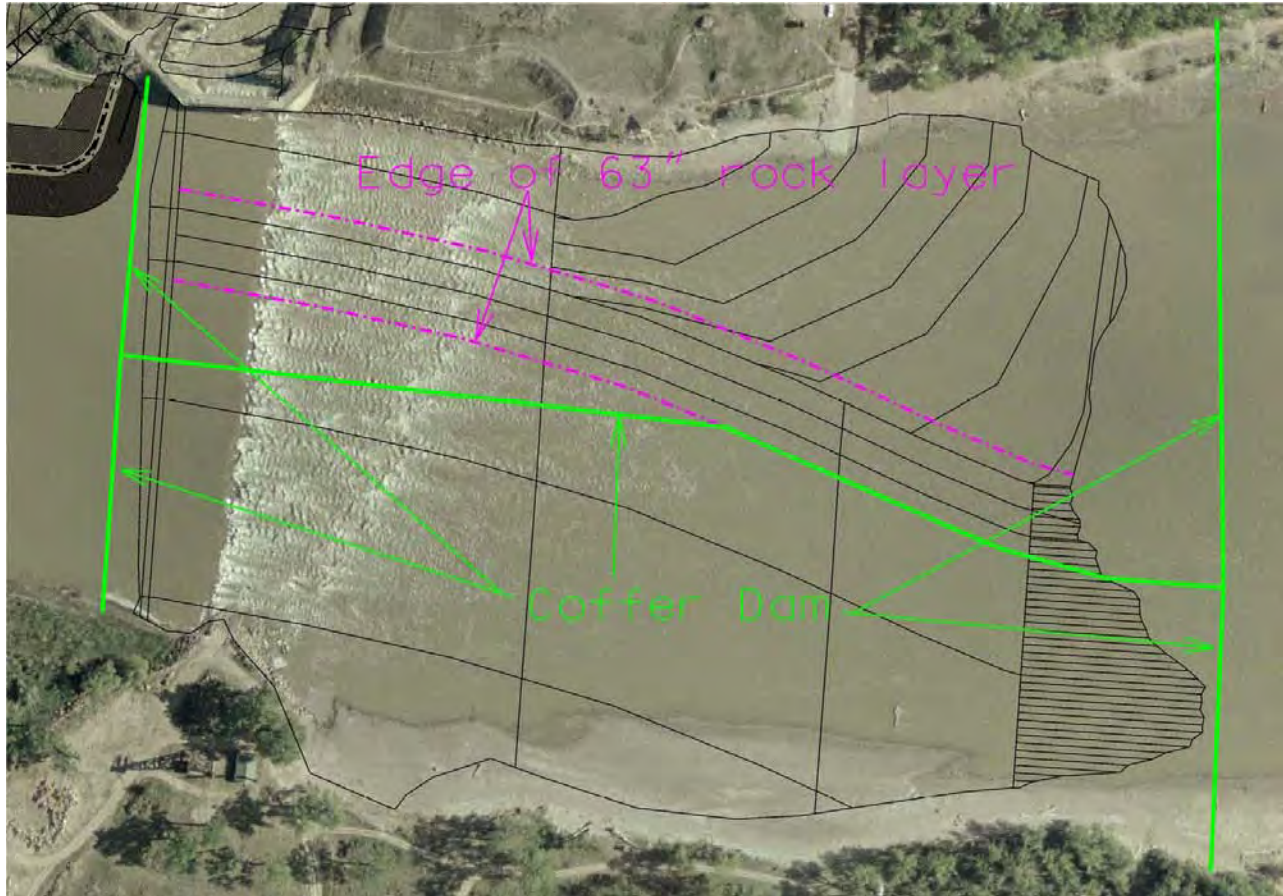
Figure 7 Half Ramp Cofferdam-General Plan (Cofferdam 3)
