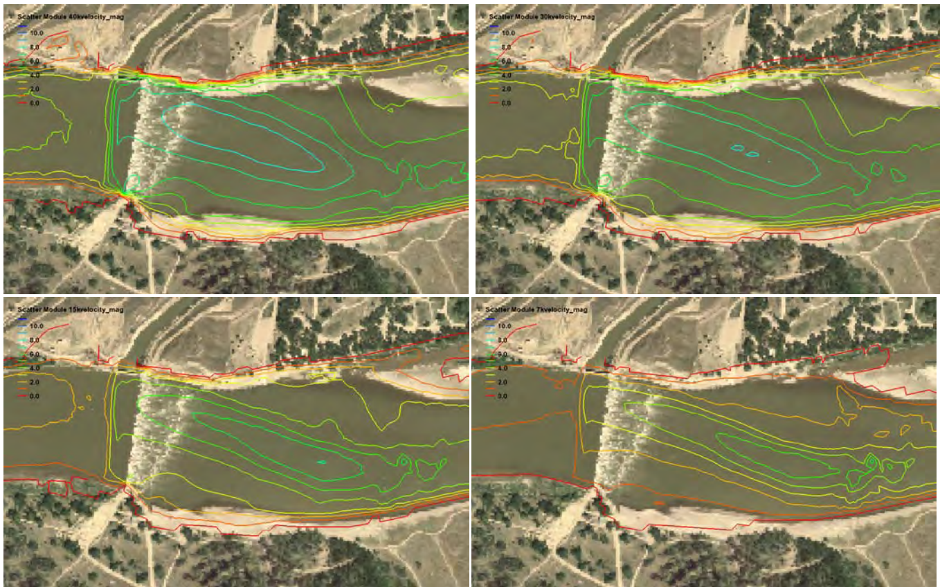
Figure 6 - Original Ramp Velocity Contours (presented in feet/second).
