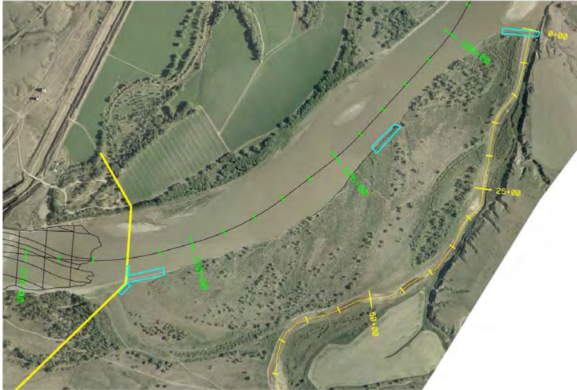
Figure 4 Grade Control and Bank Armoring Locations
