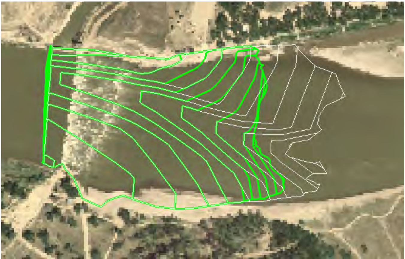
Figure 24 - 1' contours of original and Steepened Toe ramp.
