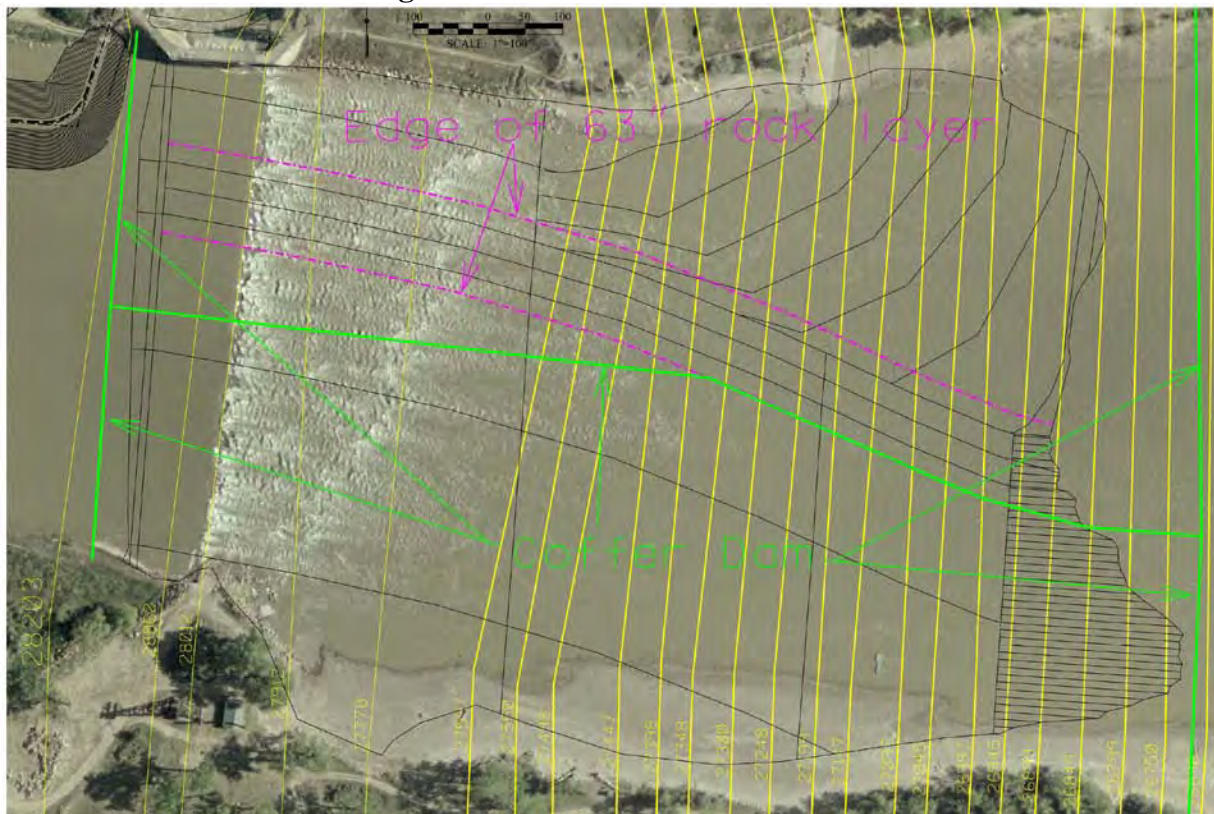
Figure 8 HEC-RAS Cross Sections
