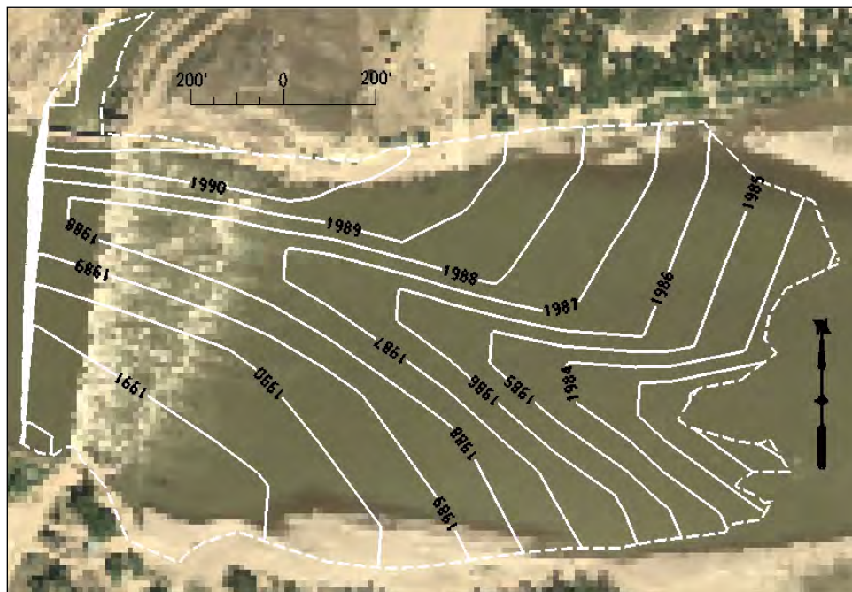
Figure 4 - Original Ramp 1' Contours
