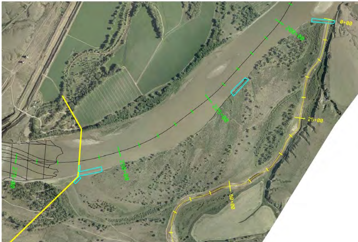
Figure 4 Grade Control and Bank Armoring Locations
