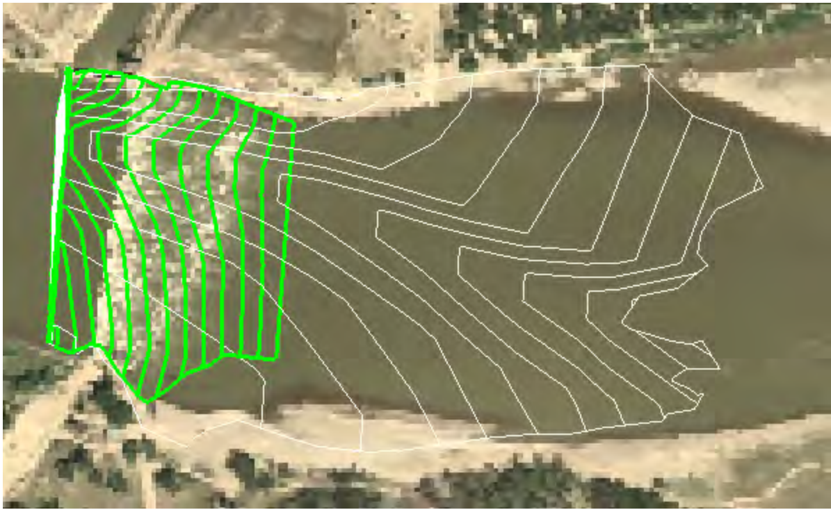
Figure 18 - 1' contours of original and Total Rock Cost Ramp.
