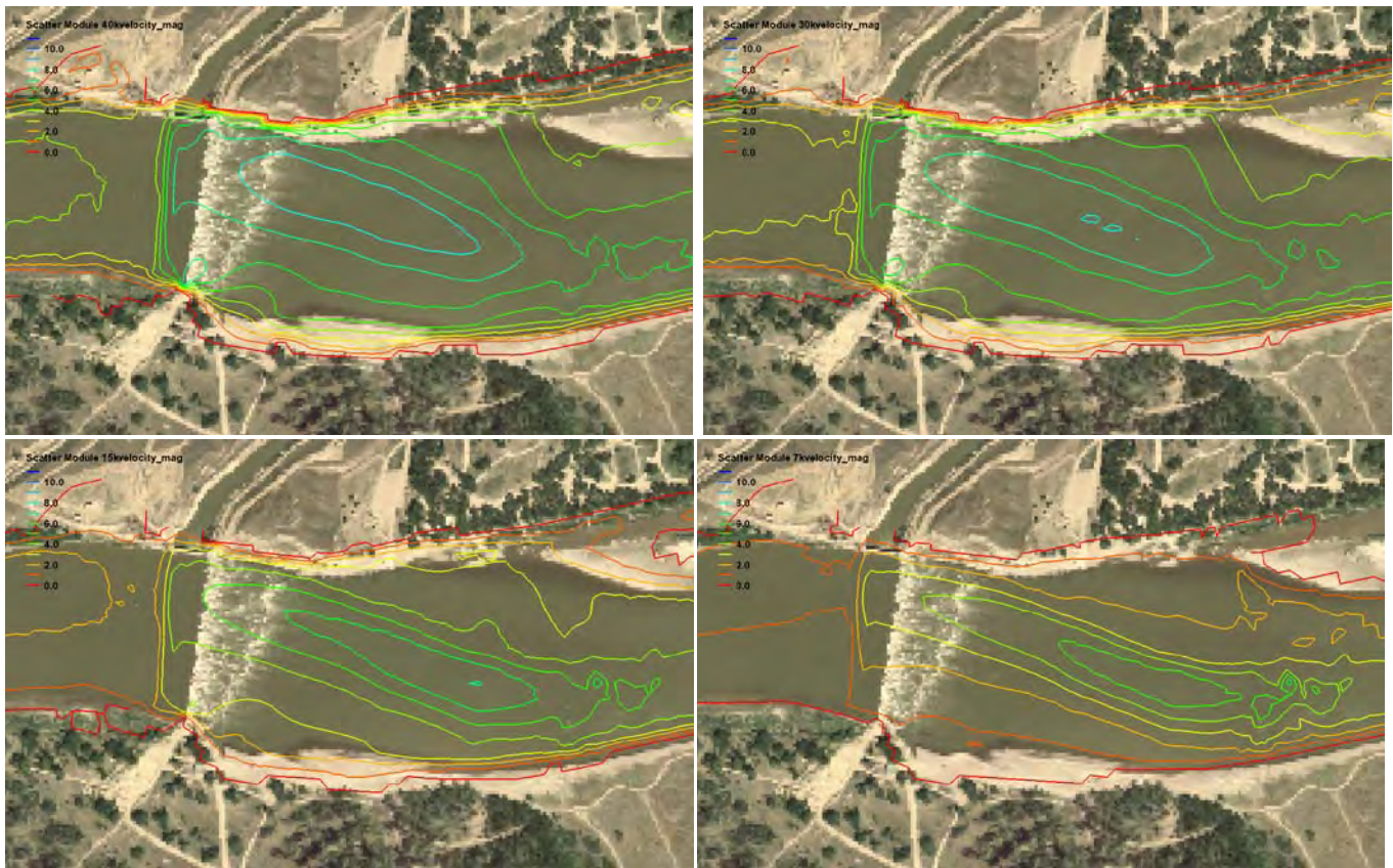
Figure 6 - Original Ramp Velocity Contours (presented in feet/second).
