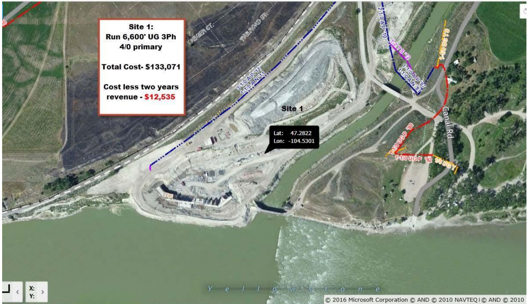
Site 1 - Power System Uprating Estimate from MDU
