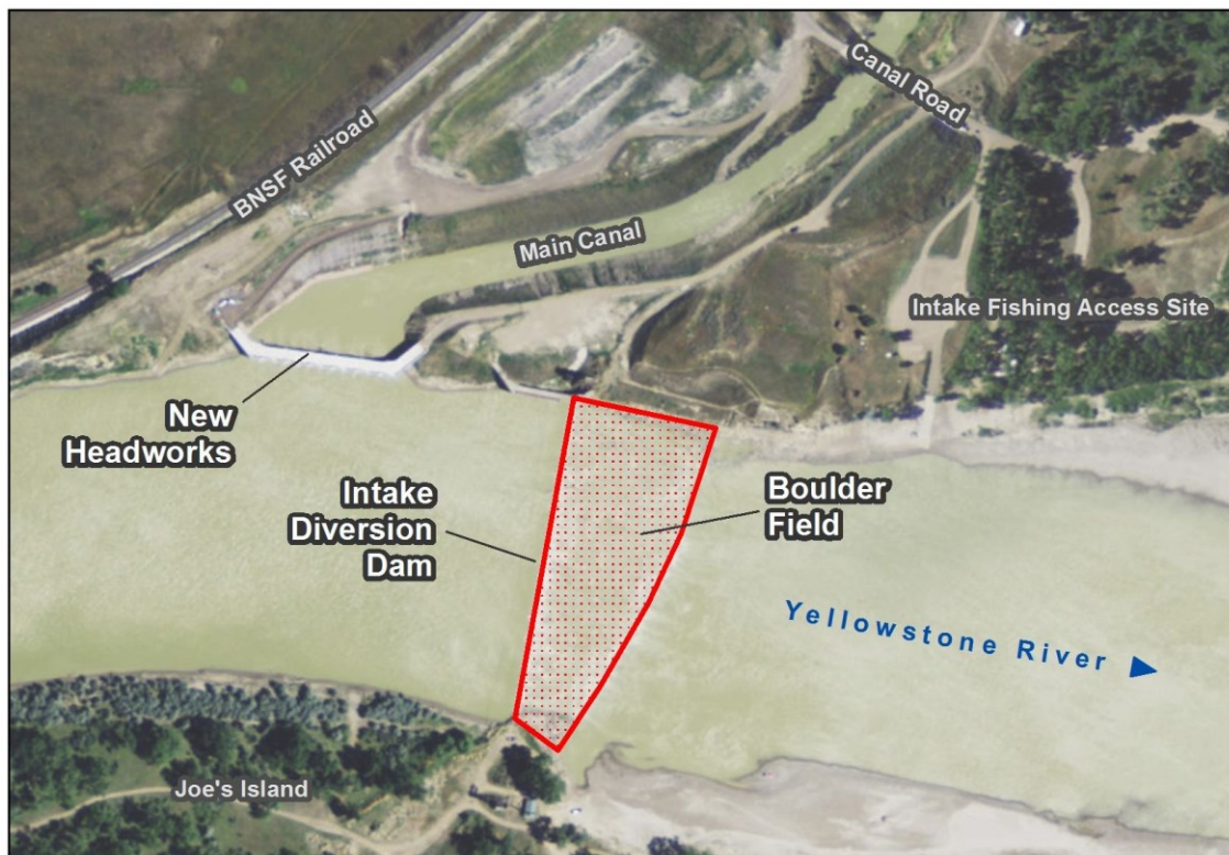
Figure 2-2. No Action Alternative with New Headworks, Intake Diversion Dam and Existing Boulder Field
