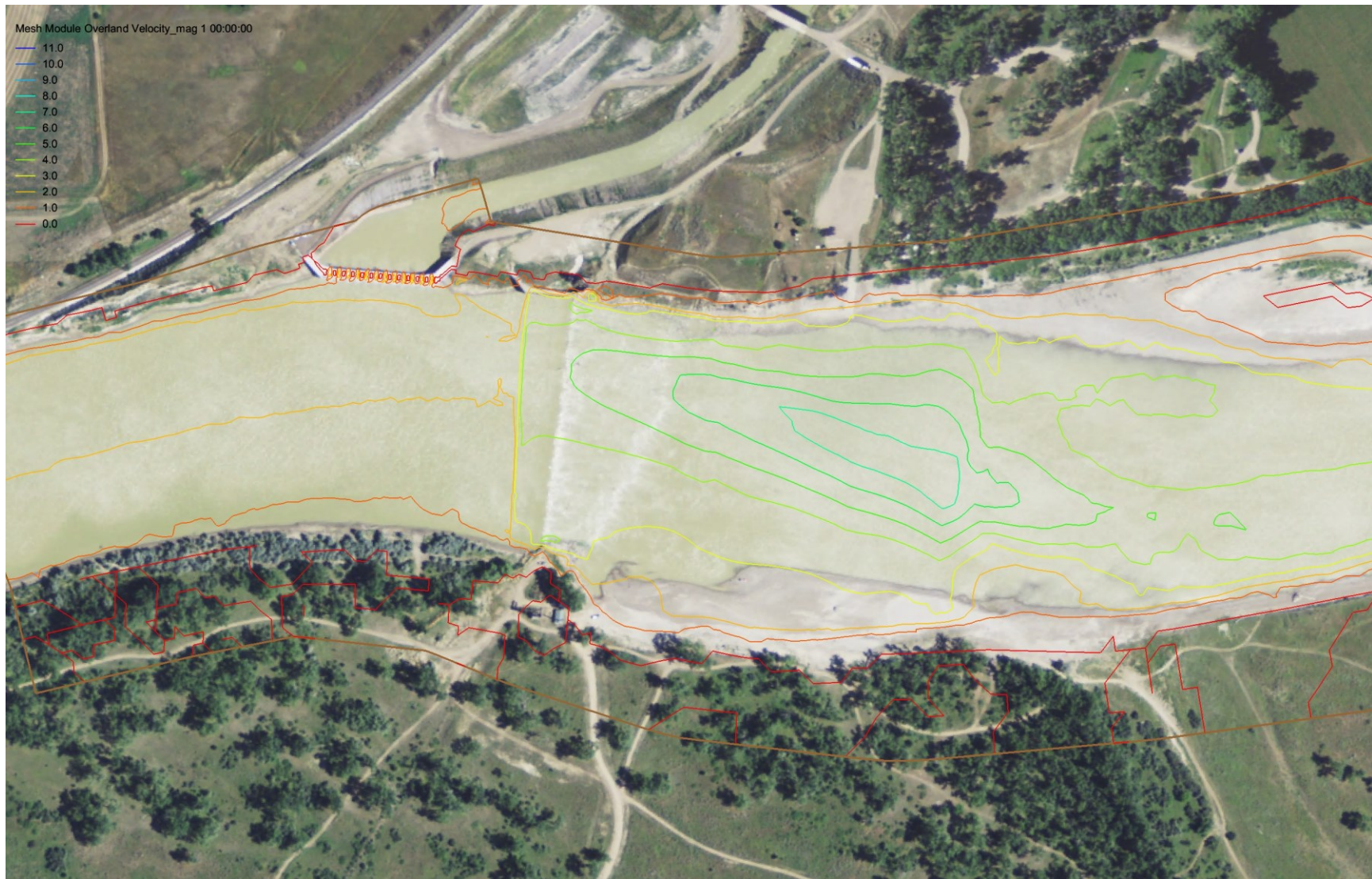
Figure 4-1. Proposed Rock Ramp Alternative Modeled Velocities at 15,000 cfs (velocity contours superimposed on aerial photo of existing conditions)
