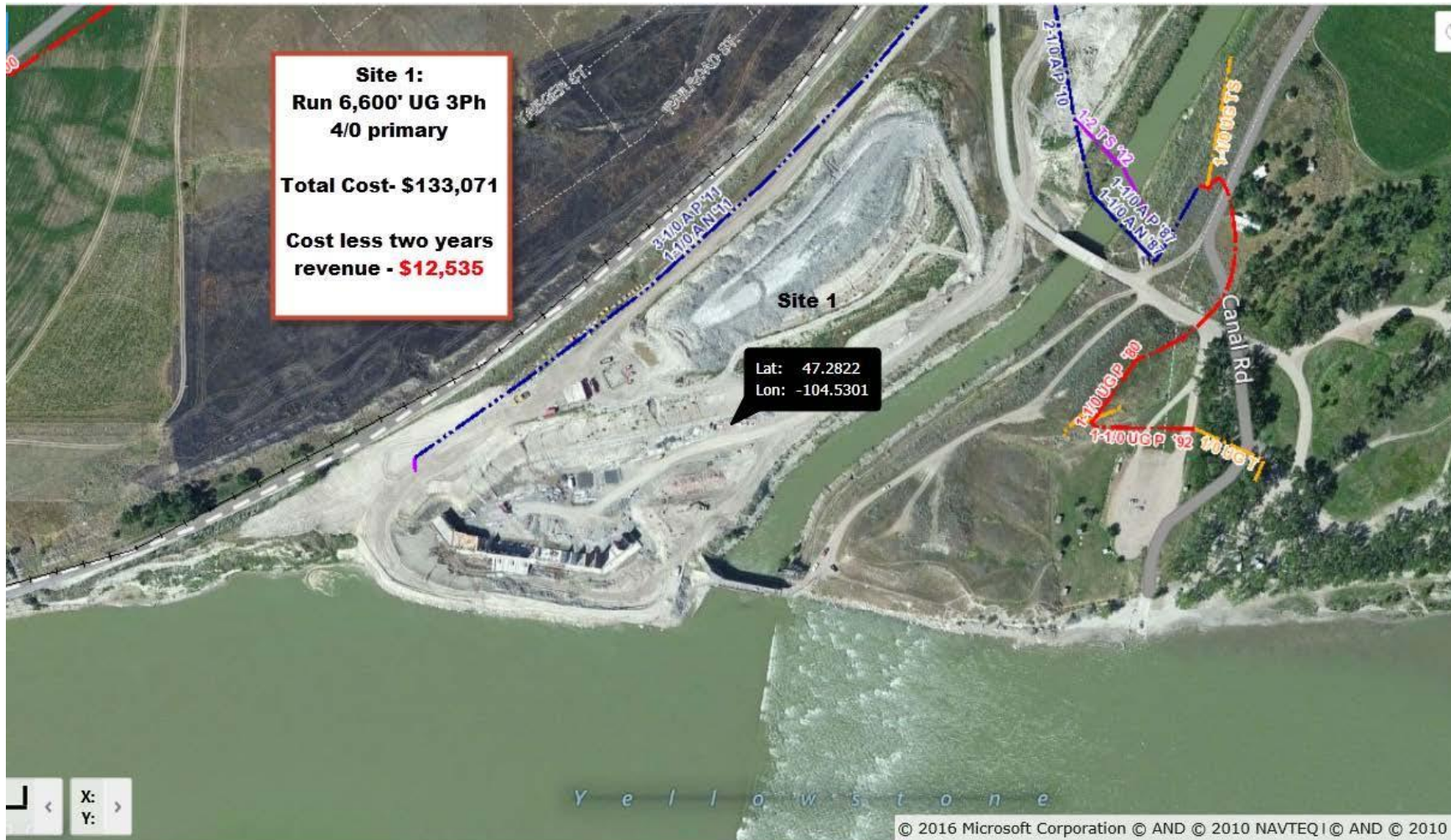
Site 1 - Power System Uprating Estimate from MDU
