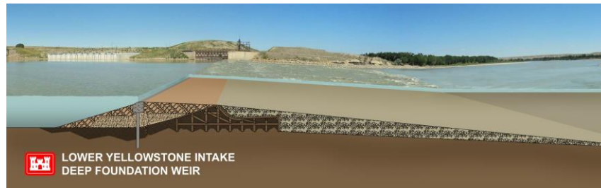
Figure 2 - Cross-section of New and Existing Weir
