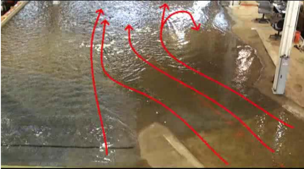
Figure 5. Fish bypass entrance flow patterns, configuration 1 (bypass invert 1983 ft), total river flow= 45,300 ft 3 /s.
