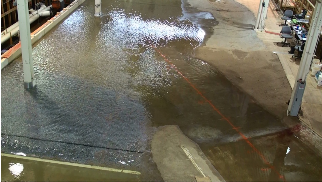
Figure 9. Physical model showing right bank topography (green shaded area) at an approximate elevation of 1990 ft. Flow is 24,000 ft 3 /s.
