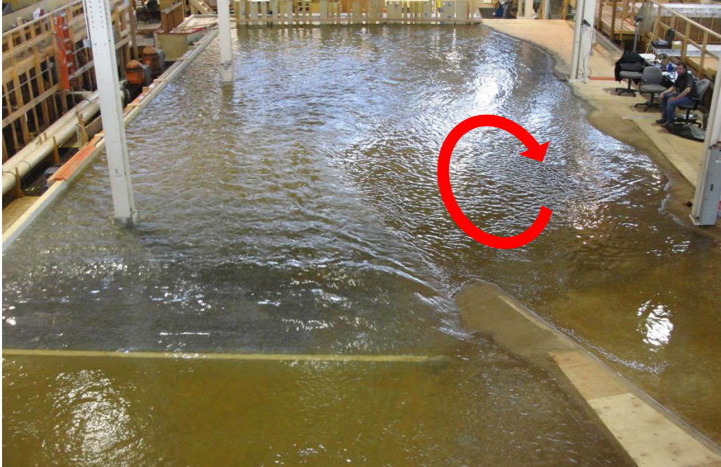
Figure 8. Physical model showing large eddy that forms on right side of river. No bypass flow. Flow is 54,000 ft 3 /s
