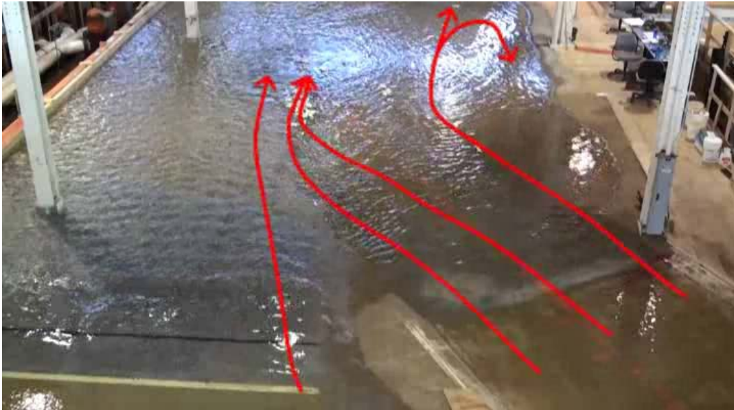
Figure 6. Fish bypass entrance flow patterns, configuration 2 (bypass invert 1981 ft), total river flow= 45,300 ft 3 /s.
