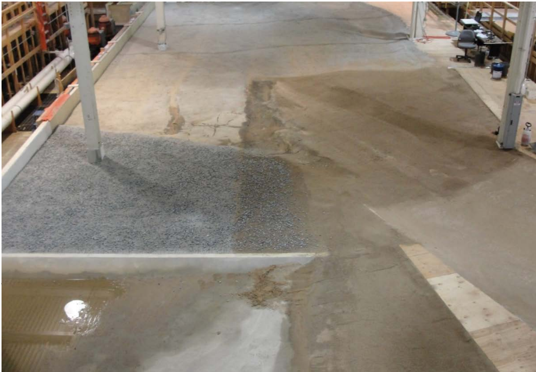
Figure 3. Picture of physical model topography looking downstream. Note only \frac{1}{2} of the river channel and dam are in the model.
