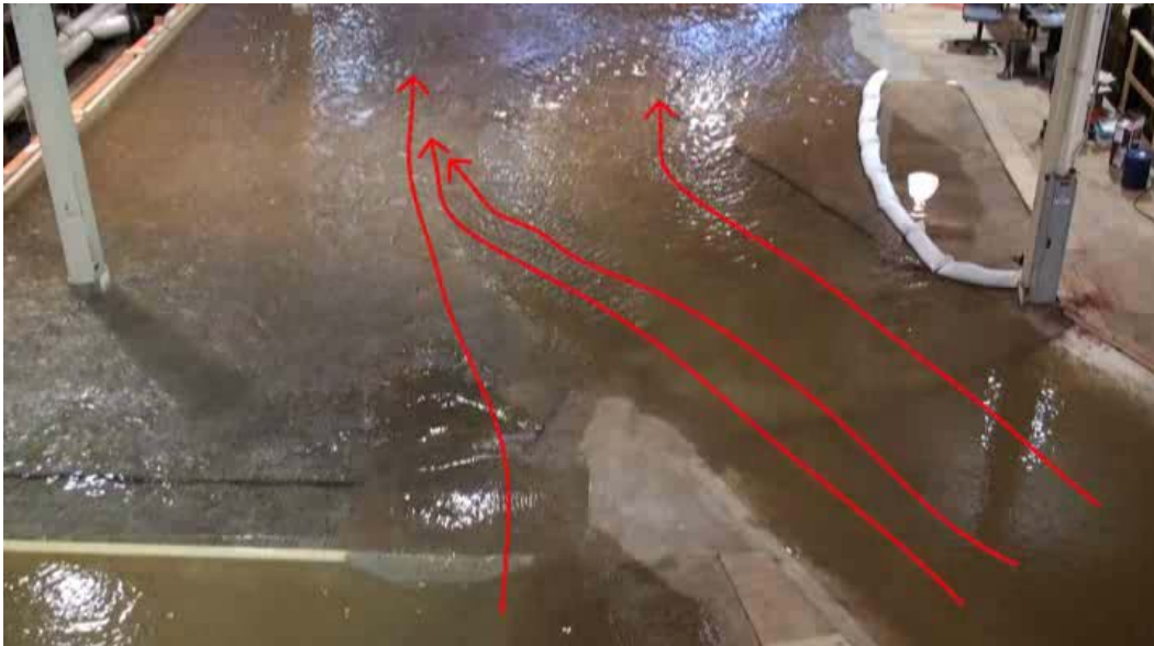
Figure 19. Fish bypass entrance flow patterns, configuration 7 (bypass invert 1981 ft, right bank topography adjustment- small, south river abutment, and notch), total river flow= 45,300 ft 3 /s
