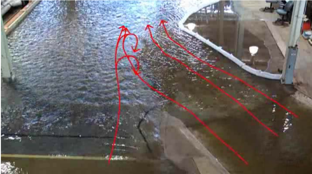
Figure 16. Fish bypass entrance flow patterns, configuration 5 (bypass invert 1981 ft, right bank topography adjustment- large, center point topography adjustment, 9% bypass split), total river flow= 45,300 ft 3 /s
