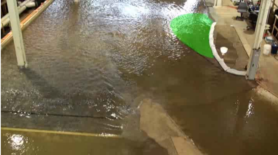
Figure 11. Fish bypass entrance flow patterns, configuration 6 (bypass invert 1981 ft, small right bank topography adjustment, south river abutment wall) total river flow= 45,300 ft 3 /s. Shaded green area represents very slow velocity.
