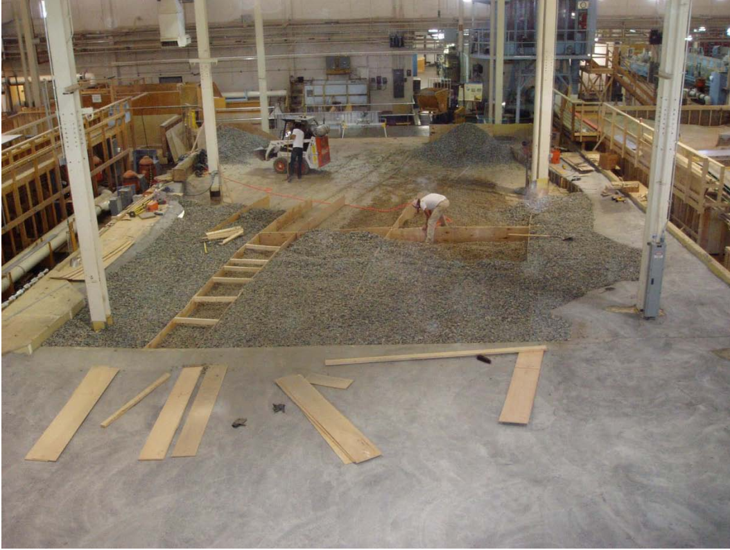
Figure D- 4. Installation of angular rock and breakline templates for model rock ramp.
