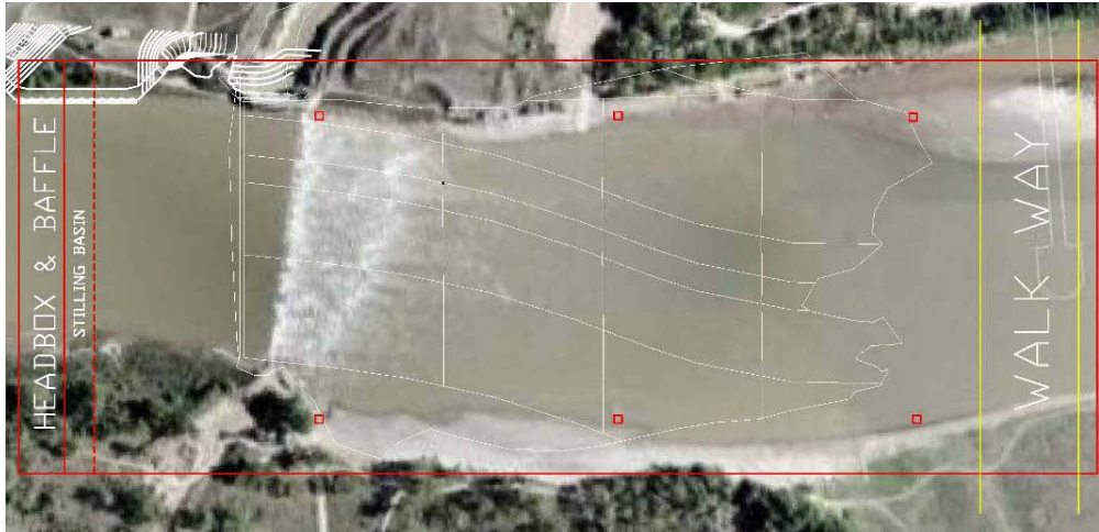
Figure 3. Extent of the 1:25 scale model of the diversion weir and rock ramp
