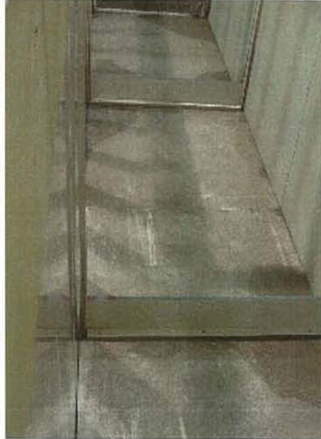
Figure 19 - View of 6 inch high weirs used to induce large scale vertical oriented eddies in the flow along the invert of the test flume.
