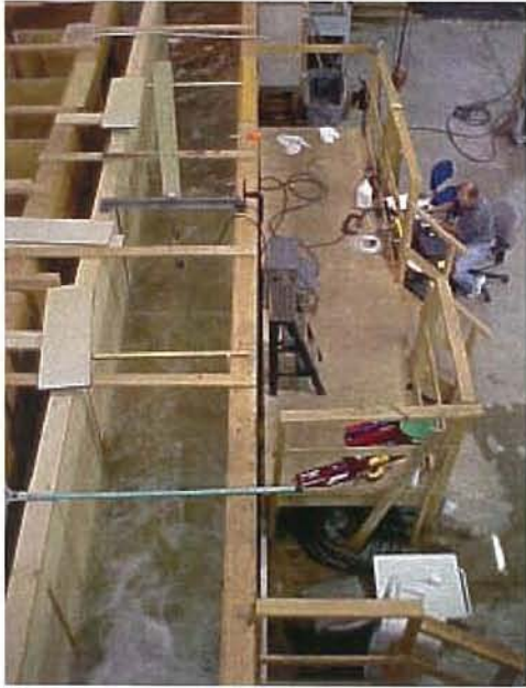
Figure 4 - View of 3 ft wide by 30 ft long by 5 ft deep horizontal flume.
