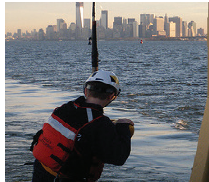
NOAA Ship Thomas Jefferson retrieves side scan sonar after surveying the Hudson River for sunken containers, debris, and shoaling that pose dangers to ships and lives.
