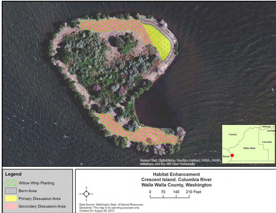
Figure 2-6. Sketch of berm and planting in the primary dissuasion area (northeast corner of island) and planting in secondary dissuasion areas.
