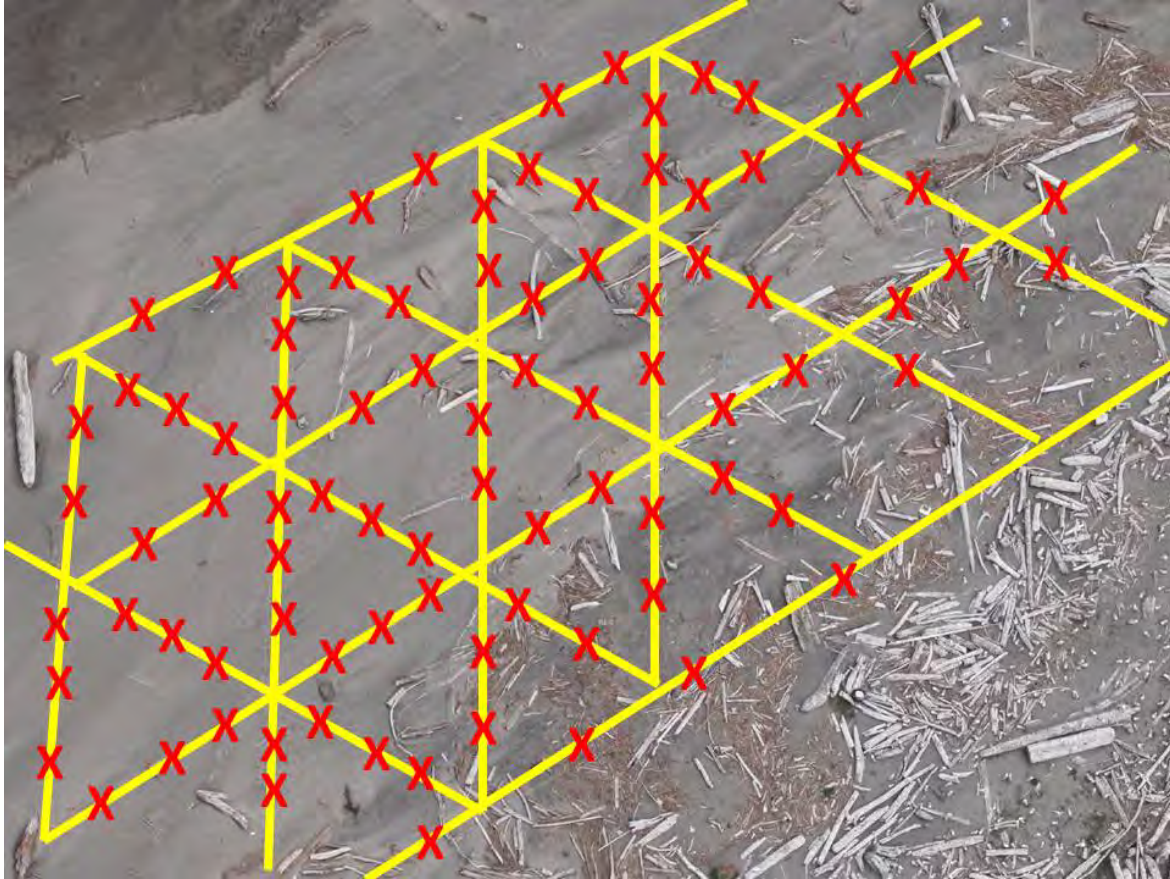
Figure 2-2. Layout of posts and flagging in the Columbia River estuary. Yellow lines designate yellow rope and a red “X” represents a length of flagging tied to the rope.
