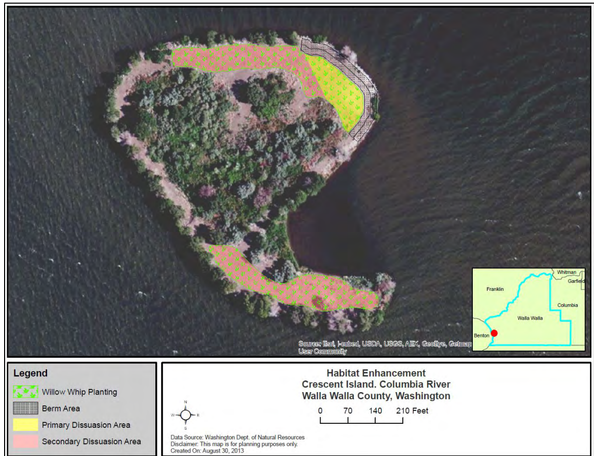
Figure 2–5. Sketch of Planting Rows in the Primary Dissuasion Area (Yellow) and Planting Rows in the Secondary Dissuasion Areas (Pink) – Excavation in the primary dissuasion area is up to 2 feet below surface level with a berm up to 4 feet high on the northeast side of the island.
