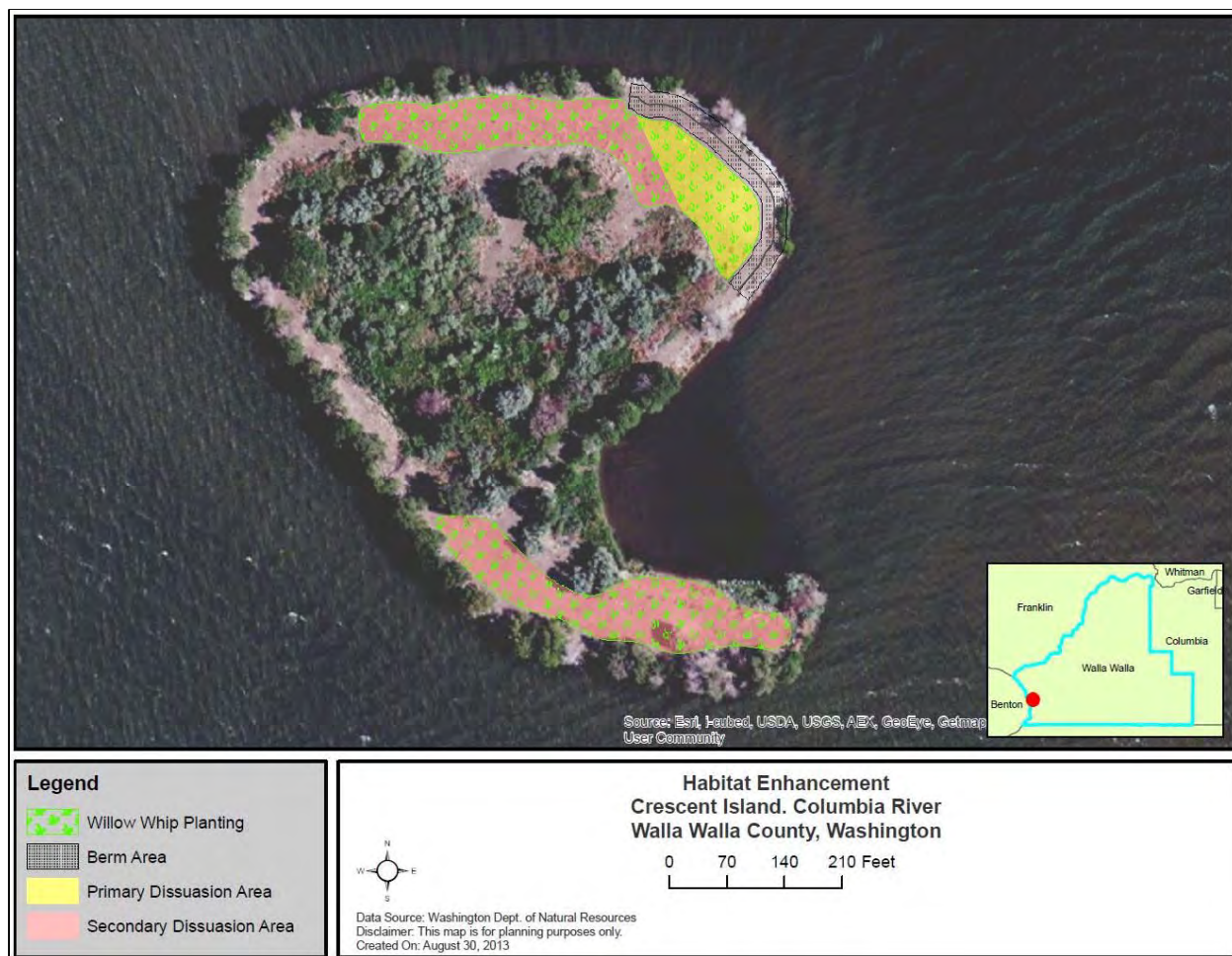
Figure 2–4. Sketch of planting rows in the primary dissuasion area (yellow) and planting rows in secondary dissuasion areas (pink). Excavation in the primary dissuasion area is up to 2 ft below surface level with a berm up to 4 ft high on the northeast side of the island.
