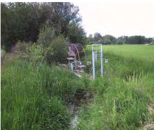
Photo 2.3-5. Nonconforming wiper-style fish screen.
