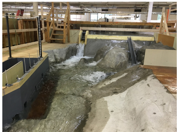
Battle Creek hydraulic model Inskip Diversion Dam fish ladder
