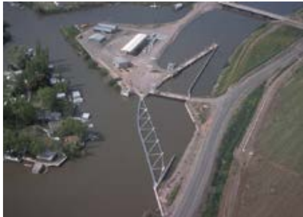
The Tracy Fish Collection Facility was constructed to protect fish natural to the area from the nearby southern Delta pumping plant.
