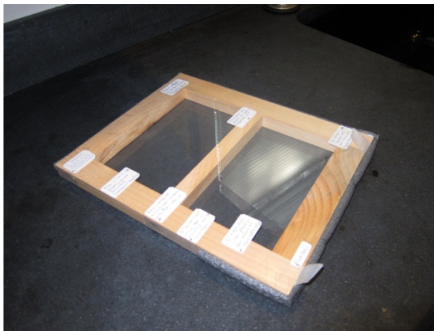
Figure 25. Interior removable storm window sample
