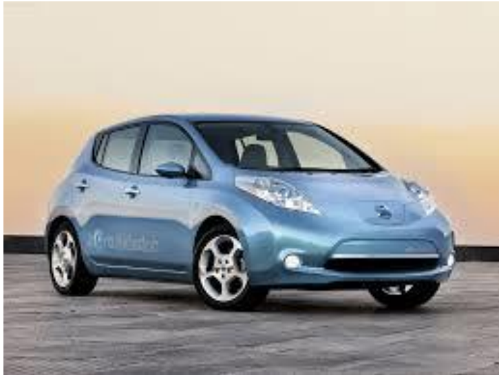
2015 Nissan LEAF 84-mile range 24 kWh battery 0.3 kWh/mile
